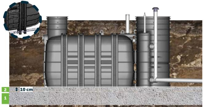
**3 -** Backfill in **30 cm increments** while **simultaneously filling the primary tank with clean water**. Compact **manually** between each slice.
