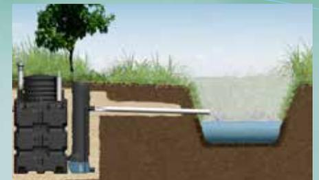
The treated water can be discharged by pump to a pressurized disposal system if required
