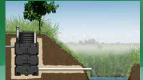
The treated water is discharged either underground (infiltration) or into a gravity disposal system depending on the ground type\*
